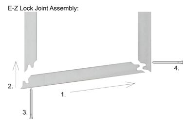
Please note the correct assembly of the E-Z Lock joint shown at the left. Nails MUST be installed only in the edges shown (3 and 4). Installing on the other edges may result in open seams.
